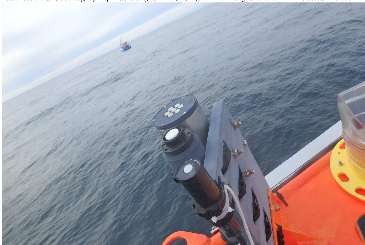
Buoy surface sensors including multispectral and hyperspectral radiometers and PAR sensor, on the top of the BOUSSOLE buoy.
